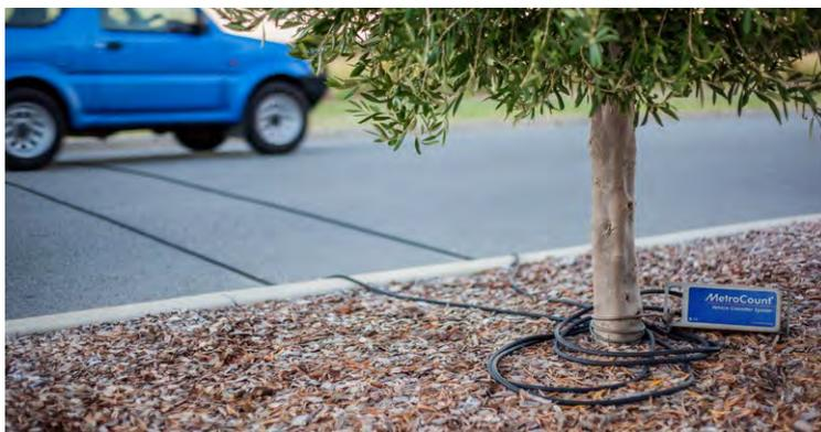
Portable counters are easy to setup and relocate.
